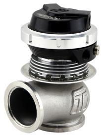
The Gen-V WG40M Comp-Gate40 Motorsport external wastegate is a cost effective, high performing 40mm external wastegate designed specifically for endurance racing or where water cooling is not available and high thermal thresholds are required for extended periods of time. The Gen-V provides extensive user configurability, world leading extended thermal performance, fatigue resistance and best in class flow performance for optimum control and longevity.
